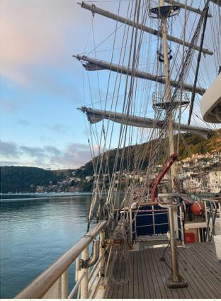
Upon nearing Dartmouth, the newly made chaffing gear was distributed forward and aft to be attached to the panamas with clove hitches. Each time we come alongside, the chaffing gear is attached because the panamas used are constantly changing.
